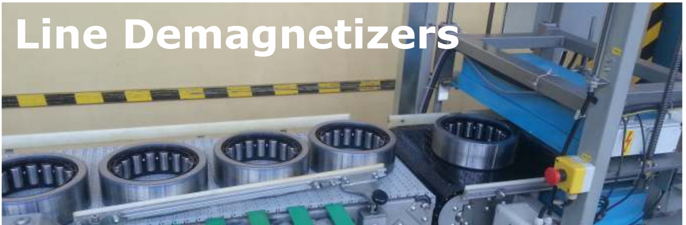
Example of using a plate demagnetizer placed in the production line for bearings.
